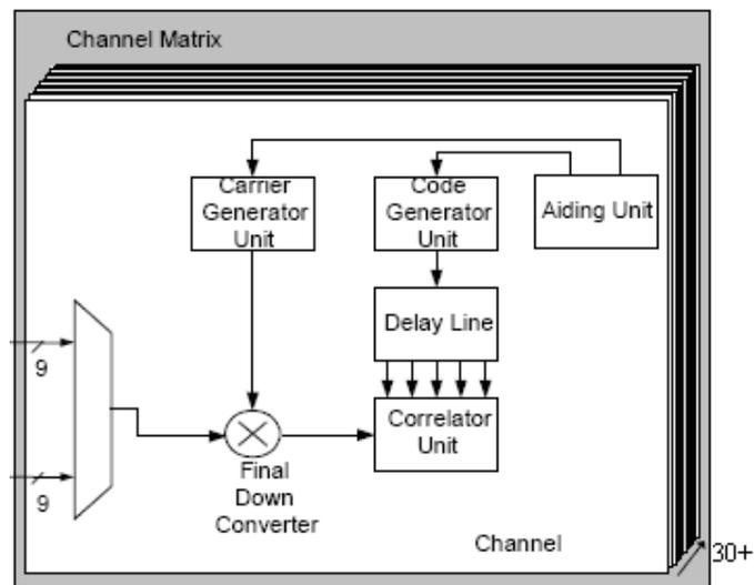
Figure 3 Functionality in the channel matrix (one of the not less than 30 channels)
