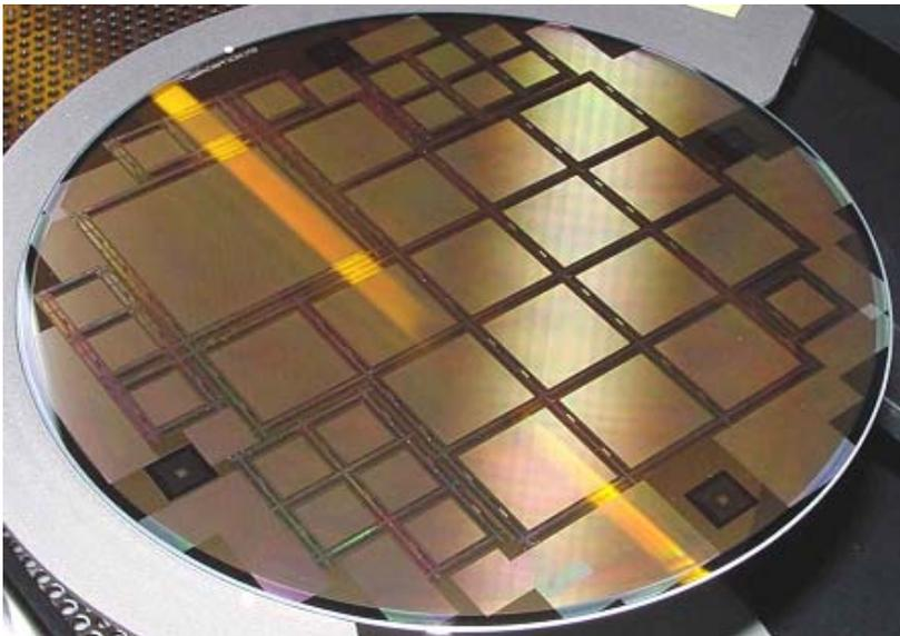
Hybrid diode array: 0.13  $\mu\text{m}$
