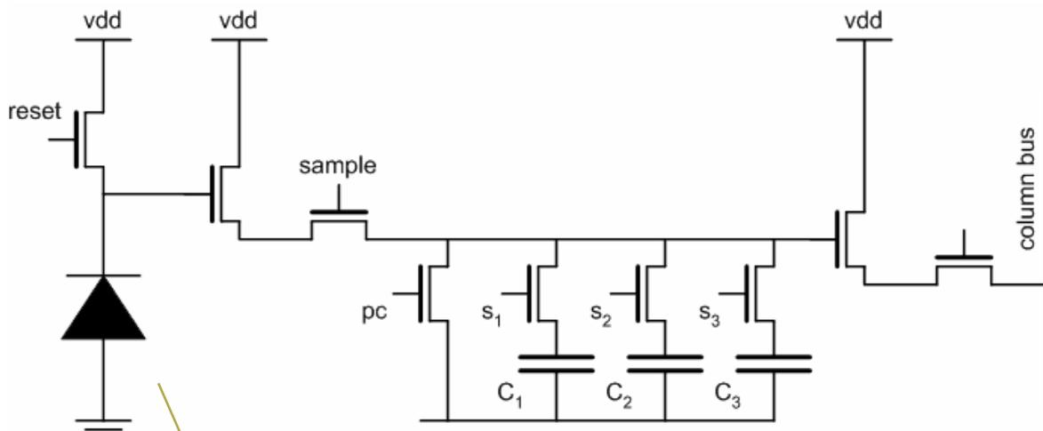
$C_{ph}$  determines charge handling capacity (FWC)
