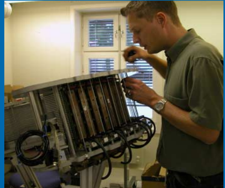
Assembly of CdZnTe based gamma camera Prototype for nuclear cardiology. 46000 channels Ideas provides complete electronic and mechanical design and assembly.
