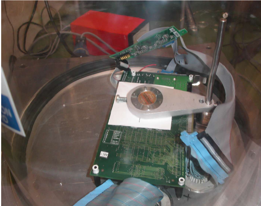
Figure 3-3: Cf-252 source placement above die cavity
