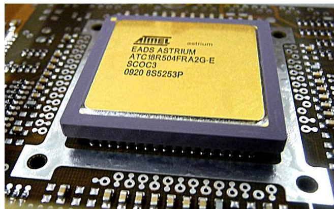
Figure 8: SCOC3 ASIC mounted on a board
