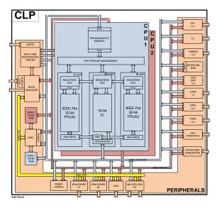
The Control Loop Processor is made of **two CPU**s (drawn in blue and read) and a number of **peripherals** (surrounded by an orange box).
