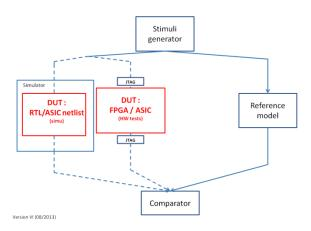
For most CLP functions, the reference model is a **cycle-accurate SystemC model**. It has been developed in parallel with the VHDL code. The SystemC model is foreseen to be integrated in the ISS as well as the various SDE tools such as the debugger of the unit test manager to take advantage of its full representativity.
