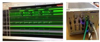
Stimuli are created by a tool generating directed stimuli and /or pseudo-random vectors according to a predefined test scenario. The stimulus then feeds the DUT and its corresponding reference model. The DUT may either be the CLP RTL code or an FPGA prototype – based on the
