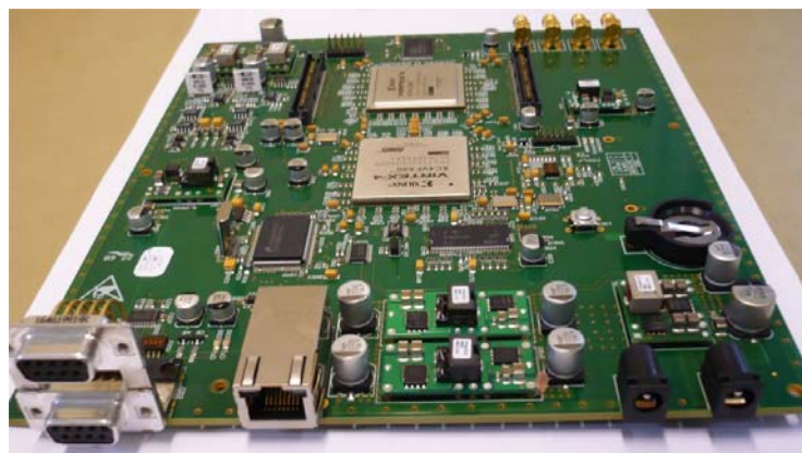
Figure 11: Assembled radiation test main board
