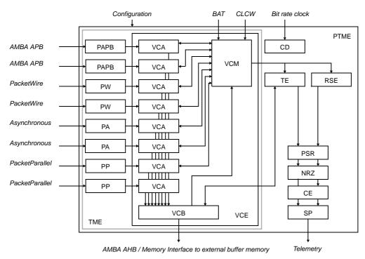
**Figure 1:** *PTME block diagram (example with eight Virtual Channels)*
