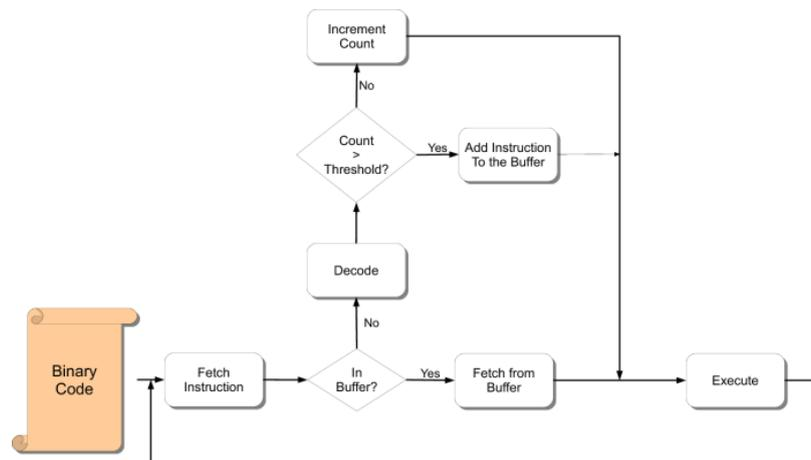
Figure 2-4: Fetch/Decode/Execute loop using the decoding buffer
