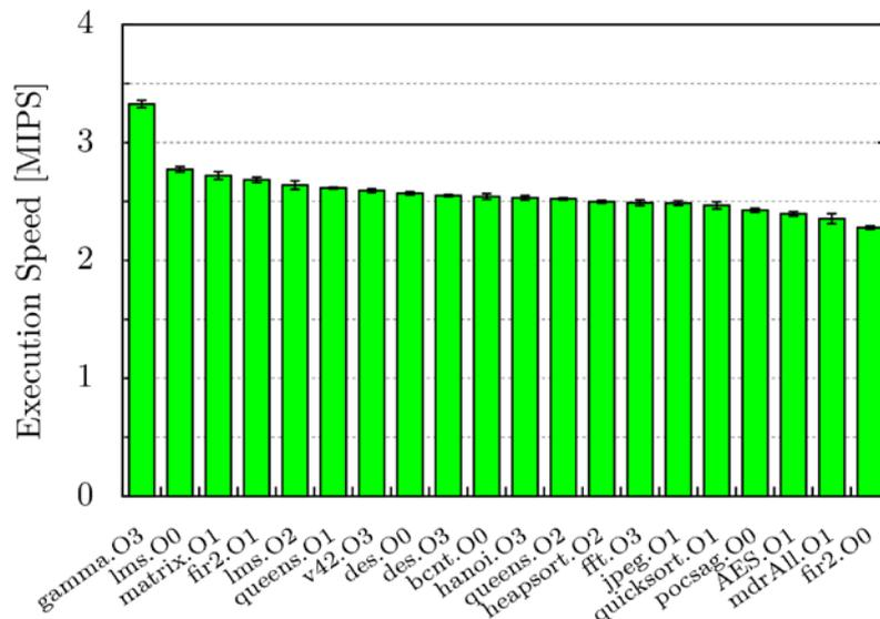
Figure 5-3: Simulation speed of the standalone Instruction-Accurate simulator with the instruction buffer disabled
