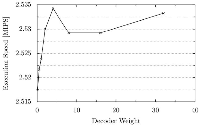
Figure 5-8: Dependence of the simulation speed from the memory weights used during decoder creation
