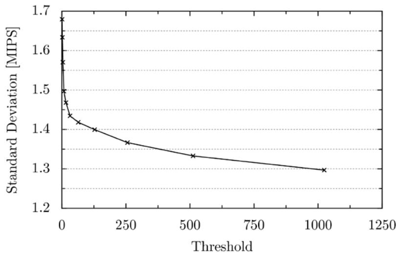
Figure 5-7: Dependence of the simulation speed standard deviation from the decoding buffer threshold  $n$
