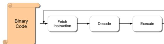
Figure 2-3: Standard Fetch/Decode/Execute loop
