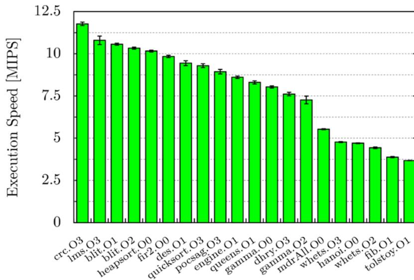
Figure 5-1: Simulation speed of the standalone Instruction-Accurate simulator with the instruction buffer enabled
