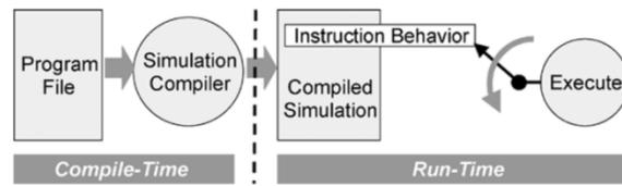
Figure 1-6: Compiled simulation cycle
