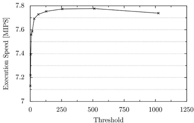
Figure 5-6: Dependence of the simulation speed from the decoding buffer threshold  $n$
