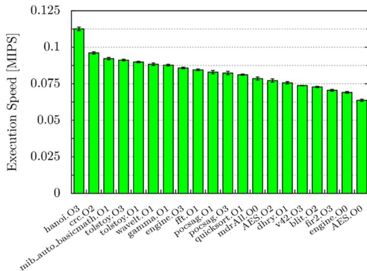
Figure 5-2: Simulation speed of the Loosely-Time Cycle-Accurate simulator with the instruction buffer enabled
