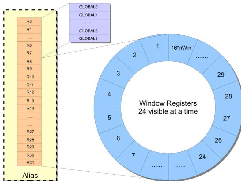
Figure 2-2: Alias mechanisms for dealing with the register windows of the LEON3 processor.
