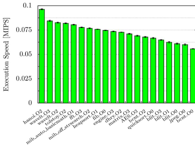
Figure 5-4: Simulation speed of the Loosely-Time Cycle-Accurate simulator with the instruction buffer disabled
