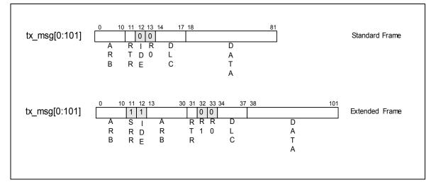
Figure 3: tx msg[0:101] structure in the case of Standard and Extended frame transmission.
