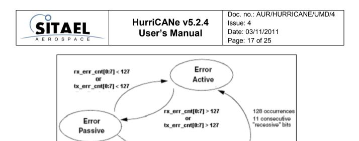
Figure 6: Error State flow diagram.
