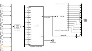
If we replace the Simulink block with a VHDL component, the rest of the system remains unchanged from the user point of view.
