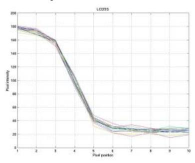
Figure 2: Pixel intensities for white to black transition on LCDSS sensor.
