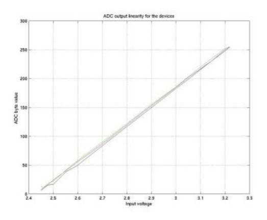
Table 17: The measured ADC output plotted against the input voltage.
