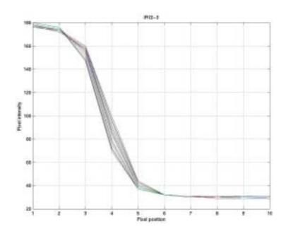
Figure 3: Pixel intensities for white to black transition on IRIS-3 sensor.
