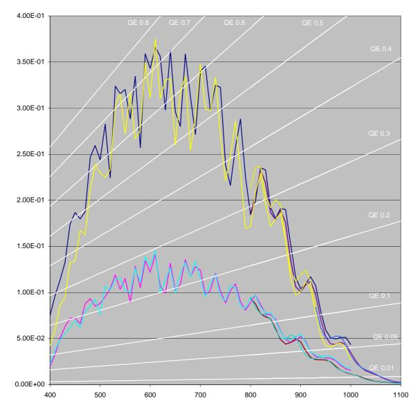
Figure 1: Spectral response measurement results as obtained with LCDSS sensor [RD1].
