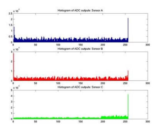
Figure 4: Histograms of ADC output levels for three sensors to detect missing ADC codes.
