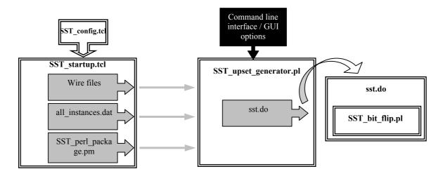
Figure 5.4 Interactions between SST\_startup.tcl, SST\_upset\_generator.pl and sst.do.
